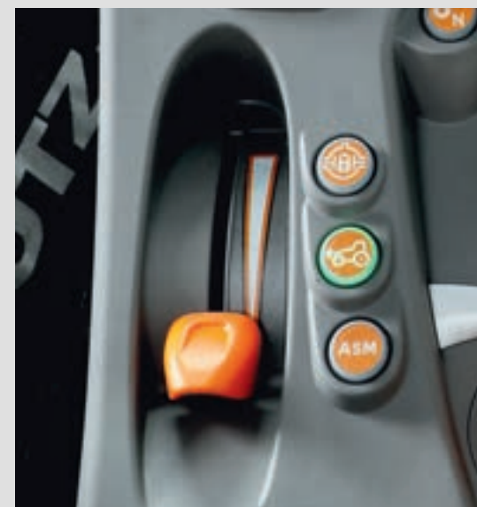
↑ Independent hand throttle and electrohydraulic activation of differential lock, all-wheel drive and ASM automatic function.
