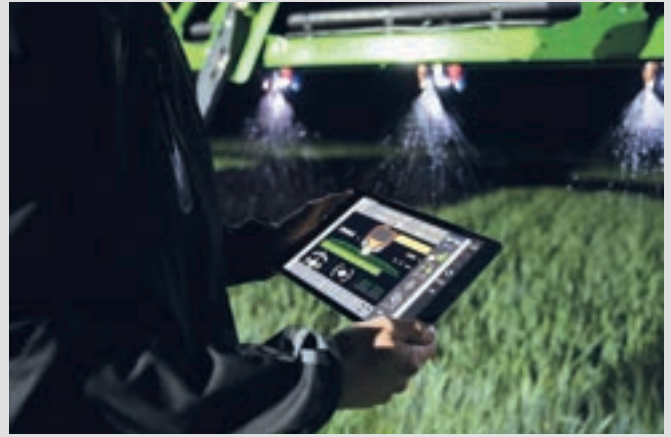
↑ XTEND function with tablet, control of implements via ISOBUS UT while being outside of the cabin.
