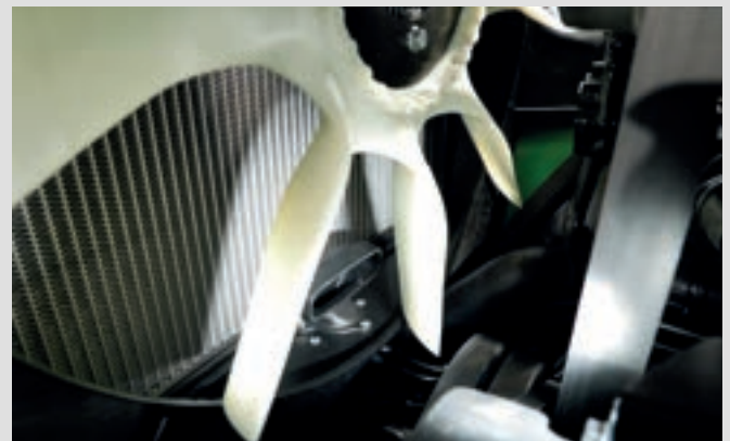
Electronic viscstatic fan (eVisco) with suction hose for air filter pre-cleaning system.
