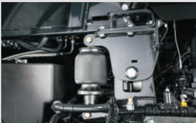
↑ Air-suspended cabin for maximum driving comfort.
