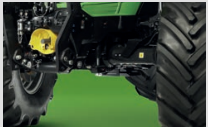
↑ Front suspension concept with high ground clearance and 3 adjustable levels inside the InfoCentre PP .
