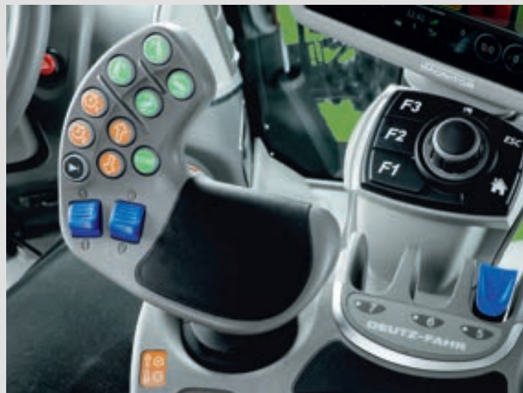
📌 Ergonomic MaxCom joystick with front and rear lift, engine, transmission, headland management and two proportional hydraulic valve control units.
